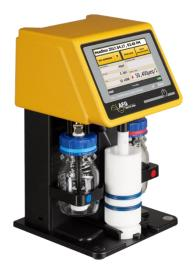
The main target of CAS measurements is to get information about the amount of anionic trash in the pulp suspension, to determine the optimal dosing of trash catcher/ fixing agent for its neutralization.
